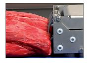
Stabilisation of the product during the slicing process makes a decisive contribution to maximum yield results. The gripper holds the product securely through to the very last slice.
