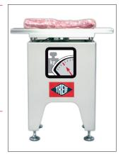
The pre-scale transmits product information to the machine to provide additional precision in cutting results. The pre-scale is optionally available in a manual version (see photo on the left) or as a continuous pre-scale.
