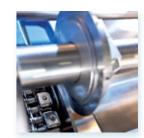
STRIP CUTTING Perfect cutting of film with powerful suction to prevent accumulation of residual strips
