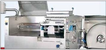
The open design ensures simple and quick cleaning. The tool changing cart (photo above) is part of the AVITOS standard equipment.
